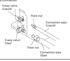
(4) When the flare nut is tightened properly by your hand, use a torque wrench to finally tighten it.
