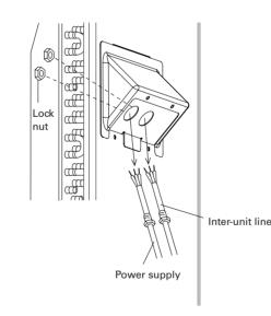
Keep the earth wire longer than the other wires
