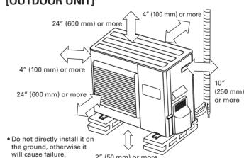
•To obtain better operation efficiency, when the outdoor unit is installed, be sure to open the front and left side
