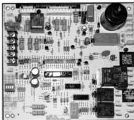
INTEGRATED FURNACE CONTROL
